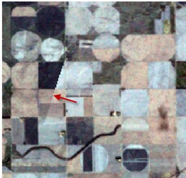
Figure 74. Showing the same masked scene that has now been filled by another scene. Notice the red arrow pointing out the boundary of where the fill scene filled the masked scene.
