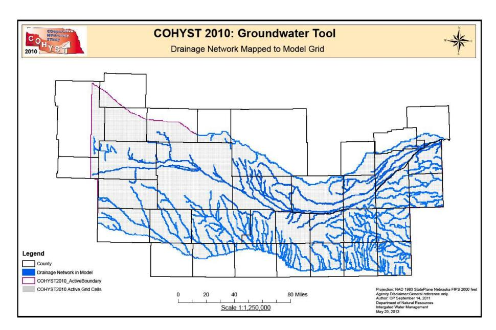
Figure 4C-2 – COHYST2010 Drainage Network Derived from Nebraska NHD and Mapped to Half-Mile Model Grid
