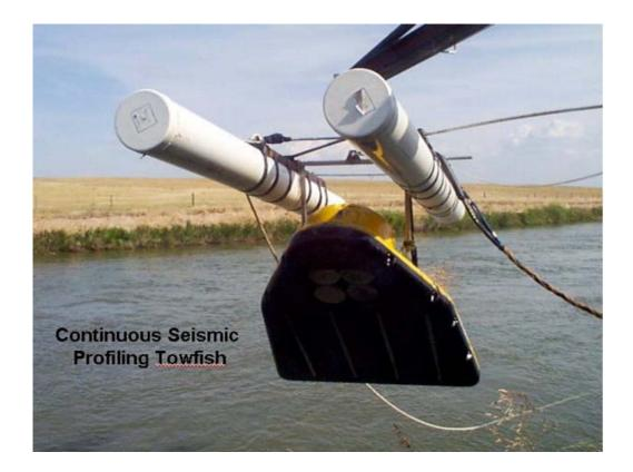
After setting the Towfish in the canal with a crane, it can be towed by two vehicles or pushed with a dinghy. Data from the Towfish is downloaded in the field to a PC and printer so that the data can be immediately verified and the instruments moved to the next study site. The effort successfully provided additional data used by COHYST's geologists for mapping the subsurface layers shown earlier.
